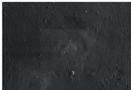
Figure 1. Scanning electron micrograph shows the distribution of silver nanoparticles (SNP) in the ointment. Magnification 10000 KX
